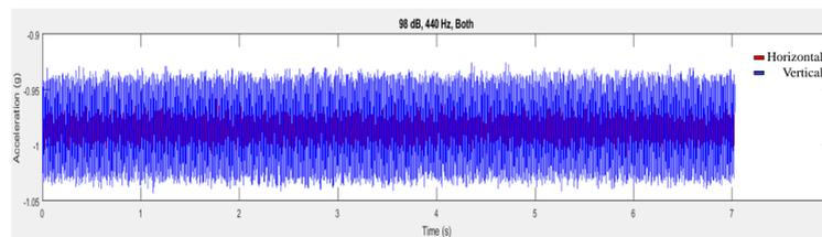
Figure 6: Signal for accelerometer data at 98 dB and 440 Hz for both block orientations
