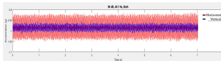
Figure 7: Signal for accelerometer data at 96 dB and 48.1 Hz for both block orientations
