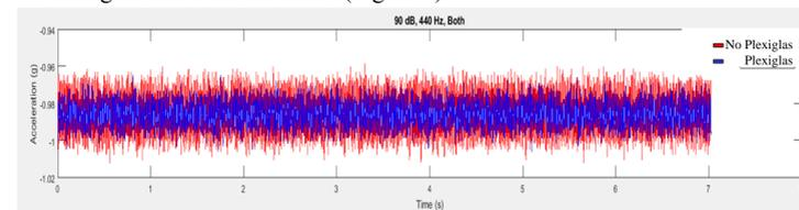
Figure 4: Signal for accelerometer data at 90 dB and 440 Hz with and without Plexiglas
