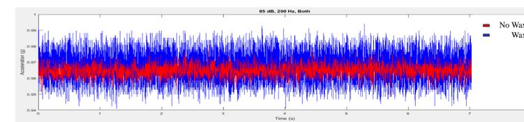
Figure 10: Signal for accelerometer data at 85 dB and 200 Hz for a fixed glass bowl
