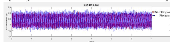
Figure 5: Signals for accelerometer data at 96 dB and 48.1 Hz with and without Plexiglas
