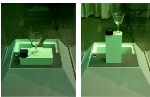
Image 3: Set-Up for horizontal and vertical block part of the speaker experiment
