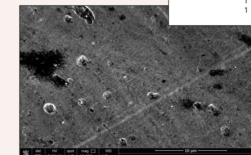
SEM micrograph of a coupon cleaned and wiped and relative EDS spectrum (Inset).
