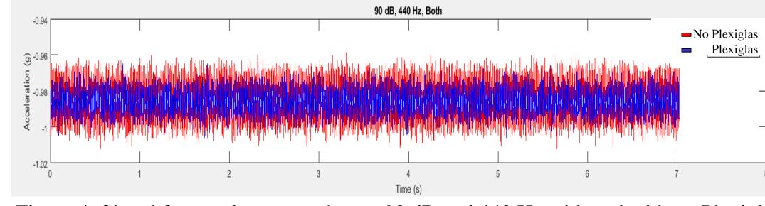
Figure 4: Signal for accelerometer data at 90 dB and 440 Hz with and without Plexiglas
