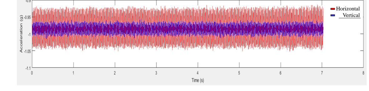
Figure 7: Signal for accelerometer data at 96 dB and 48.1 Hz for both block orientations
