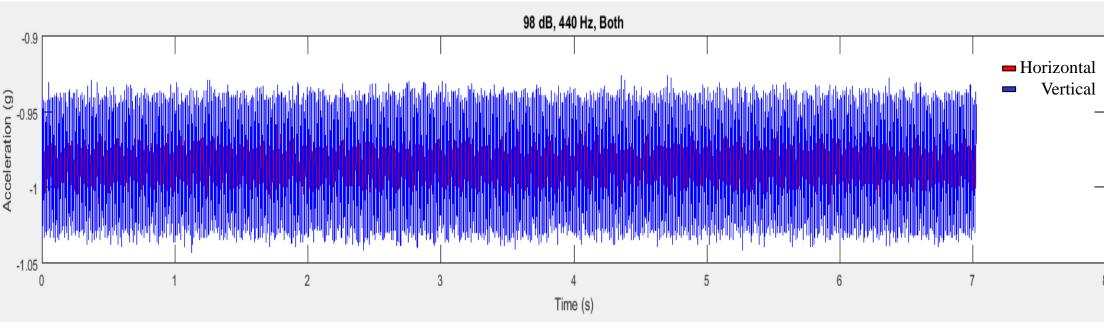
Figure 6: Signal for accelerometer data at 98 dB and 440 Hz for both block orientations
