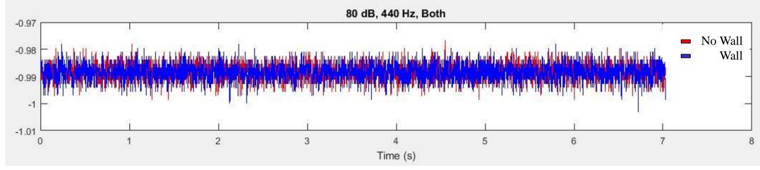
Figure 9: Signal for accelerometer data at 80 dB and 440 Hz for the display case against the wall and freestanding
