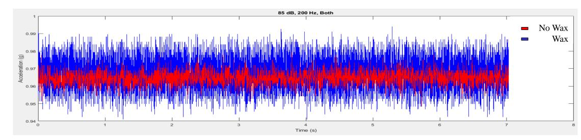
Figure 10: Signal for accelerometer data at 85 dB and 200 Hz for a fixed glass bowl
