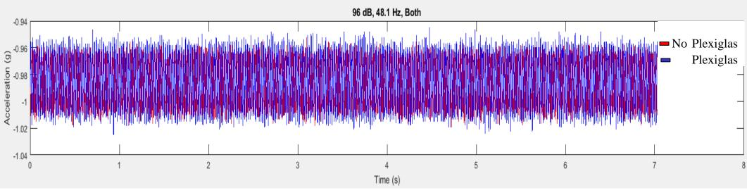
Figure 5: Signals for accelerometer data at 96 dB and 48.1 Hz with and without Plexiglas
