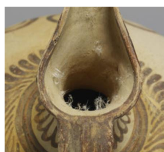
Crystals forming on ceramic piece due to exposure to formic Acid The Walters Art Museum Part 11051
