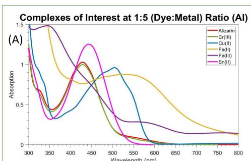
**Figure 3 (A)** The absorption spectra of Alizarin and metals which created the most change when the ratio of metal to dye was approximately 1:5 (Alizarin: Metal)
