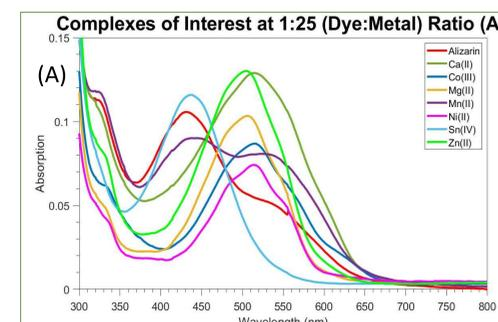
**Figure 4 (A)** The absorption spectra of Alizarin and cations which created the most change when the ratio of metal to dye was approximately 1:25 (Alizarin: Metal)
