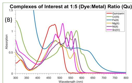
**Figure 3 (B)** The absorption spectra of Quinizarin and metals which created the most change when the ratio of metal to dye was approximately 1:5 (Quinizarin: Metal)
