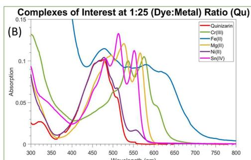
**Figure 4 (B)** The absorption spectra of Quinizarin and cations which created the most change when the ratio of metal to dye was approximately 1:25 (Quinizarin: Metal)
