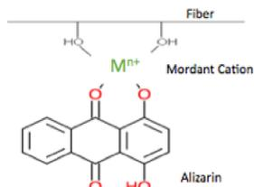
**Figure 1:** Chemical complex between textile, mordant, and pigment (alizarin). Possible coordination complex between metal salt in mordant and dye is shown.
