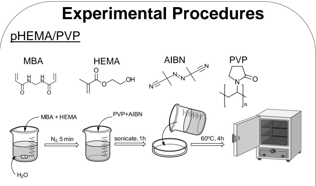
Fig.5. Synthesis of pHEMA/PVP hydrogel. The procedure was adapted from ref.[4]. The hydrogel was synthesized either with 20% w/w HEMA (HEMA 20) or 5% w/w HEMA (HEMA 5).
