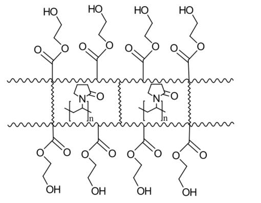
Fig.3. The chemical structure of pHEMA/PVP hydrogel.
