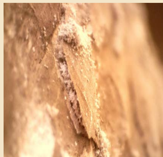
Fig. 1: Microscopic image of flaking on Egyptian limestone artifact.
